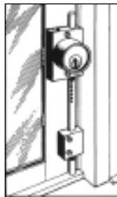
Installation at base of sliding patio door
